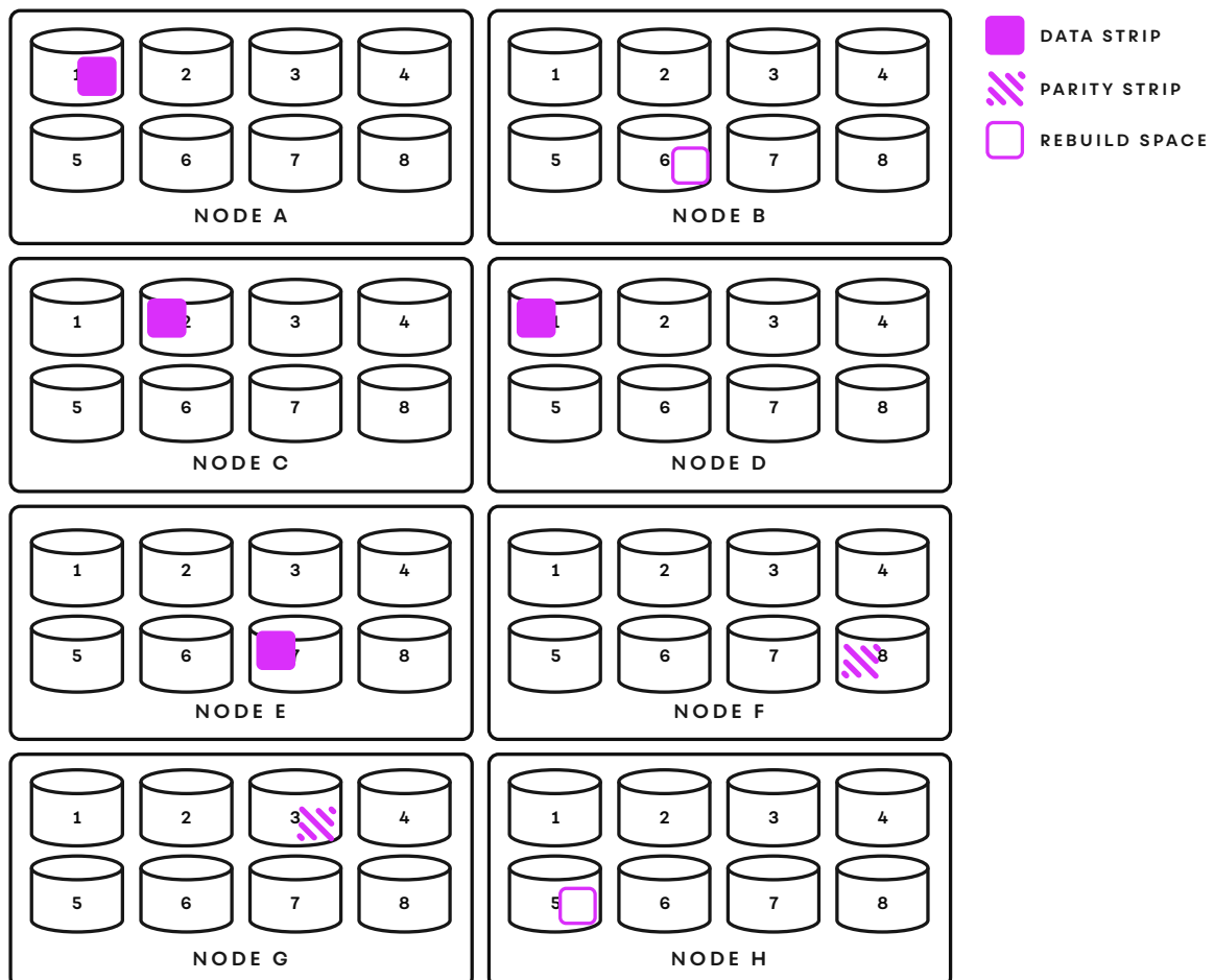
Figure 1 shows how a shared-nothing system would lay out a double-parity data stripe.
